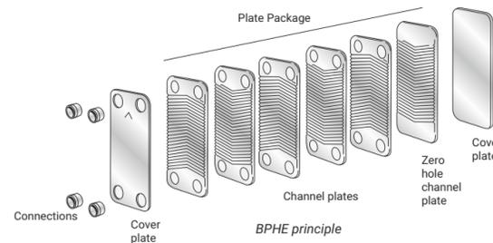
The fluids can pass through the heat exchanger in different ways. For parallel flow BPHEs, there are two different flow configurations: co-current or counter-current.
